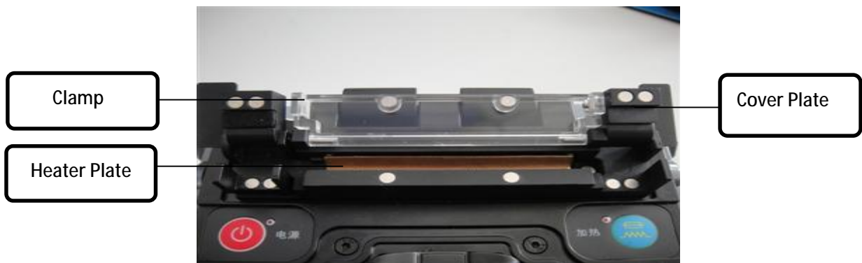
Figure 1-4 Tube Heater Structure
