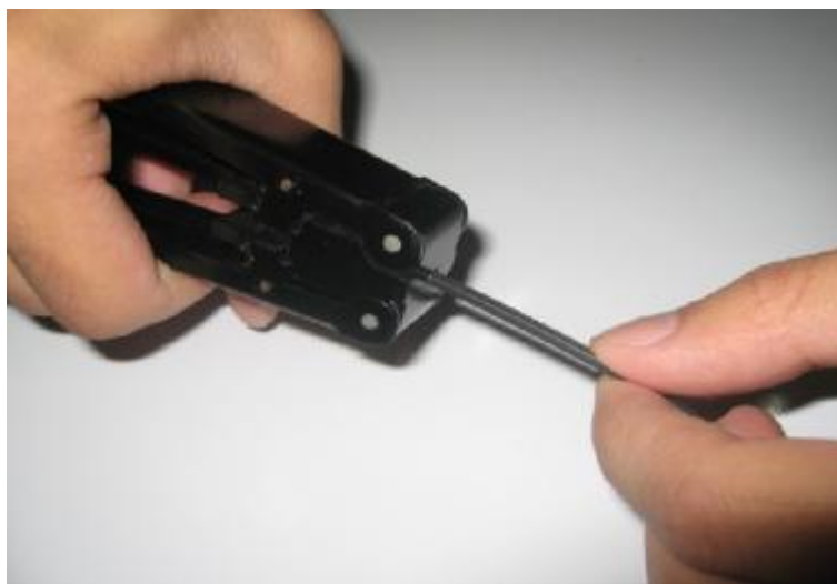
Figure 2-6 Butterflyed Fiber Strip
