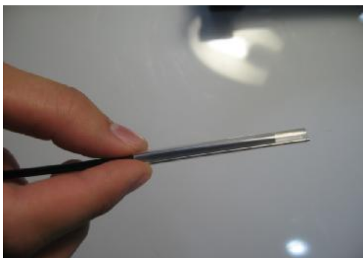
Figure 2-8 Placing Protection Sleeve
